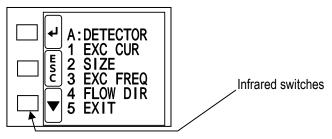
(4) Switch position : **RIGHT** The infrared switches are located at right with the front facing you.
